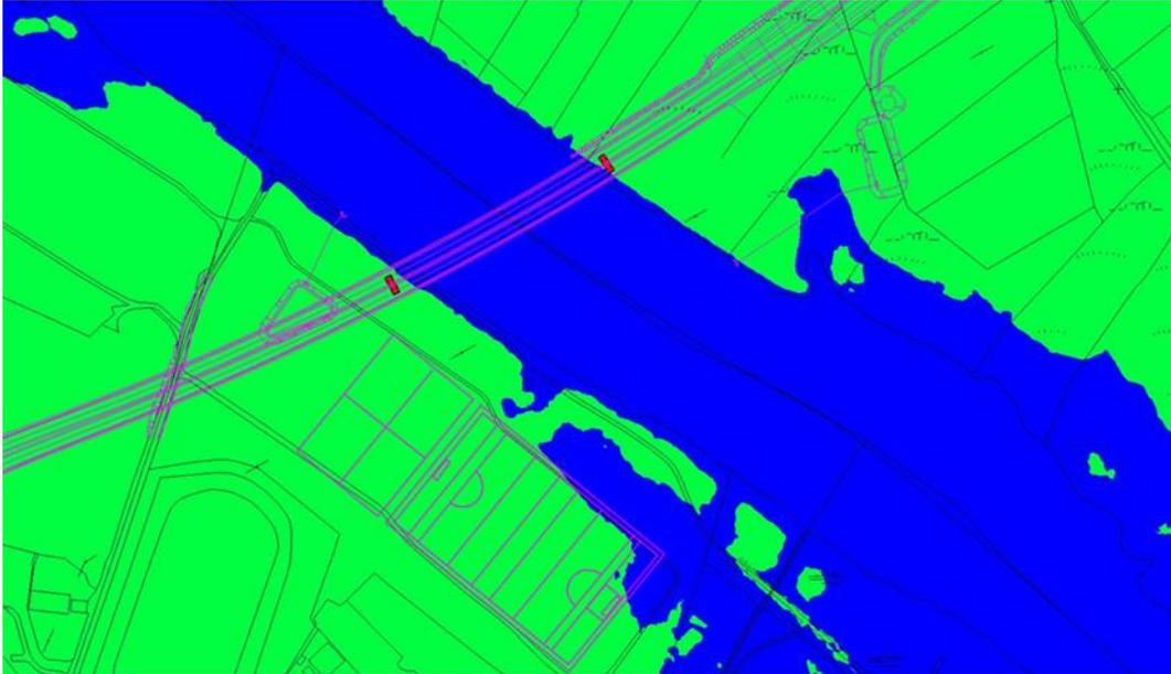
In order to avoid any potential scour risk associated with the construction of these bridge structures, abutments for bridges will be sufficiently set back from the channel bank edge with foundations located at depth. This will protect the river channel from changes in morphology whereby the channel over time would naturally migrate towards one of the abutments.
